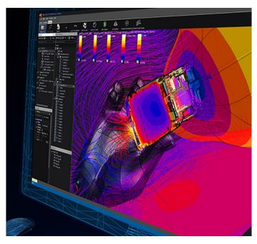
The Electromagnetics Full Wave Solvers (P-EM-FDTD) enable accelerated full-wave, large-scale EM modeling (> billion voxels) using Yee discretization on geometrically adaptive, inhomogeneous, rectilinear meshes with conformal sub-cell correction and thin layer models, offering support for dispersive materials. The solvers also include many unique features for EM safety assessments (see IMSAFE).
