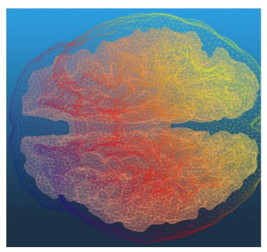
Adaptive, rectilinear meshes (e.g., for P-EM-FDTD, P-ACOUSTICS, P-THERMAL) can be generated interactively with excellent heuristics-based automatic grid generation and flexible tuning.
