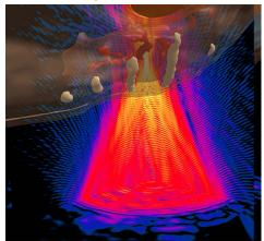
The novel ultrasound solvers account for pressure wave propagation, density variations and jumps, non-linearity, and diffusivity losses that occur in human tissue.
